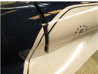
☐ Lower main landing gear by opening the gear doors and removing wire ties, the landing gear will push out and lock.
