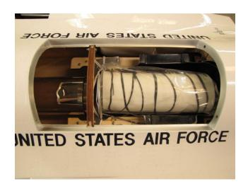
☐ Remove the rear wire tie securing the tail pipe.
