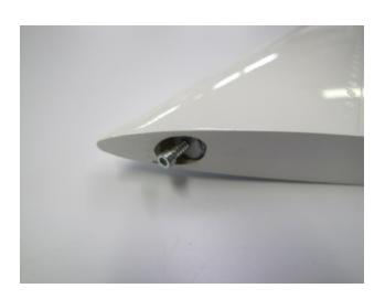
☐ Apply polyester putty, before it totally cures, trim excess with a razor. Touch-up paint with the appropriate Model Master paint and brush.
