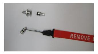
☐ Install the fittings to your overflow/taxi tank. Use an overflow tank while fueling to prevent spillage and to ensure fuel tanks are full before flight.
