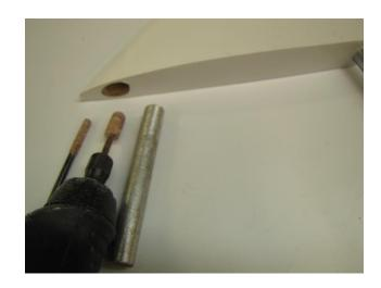
□ Prior to inserting the rod into the stab, drill a 5/64" hole about 3/8" deep into one end of the lead rod. Partially insert a servo mounting screw that will serve as a handle to maneuver the rod while gluing it into the stab.
