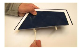
☐ Gently install the ventral fins, a rocking motion may help. Use a 3/32 hex driver to snug the internal clamp that retains the fins.
