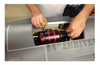
☐ Plywood rails were notched as shown to clear the KingTech engine mount.
