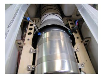
☐ Make openings in the bypass and cover for the fuel and electrical connections.
