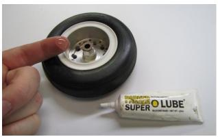
☐ Apply Super Lube BVM #5784 into the wheel bushings.
