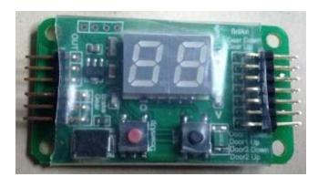
programmed with sequencing delay. See the section titled "Landing Gear/Door /Brake Sequencer Instructions" if adjustments are required. The set of two valves are connected to the gear doors, open and closed. The set of three are connected to the landing gear; Brakes,
