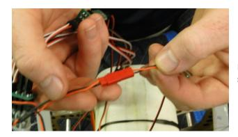
☐ Connect the Red connector for the nose gear landing light. All 3 landing lights should be connected to the "tri-harness".
