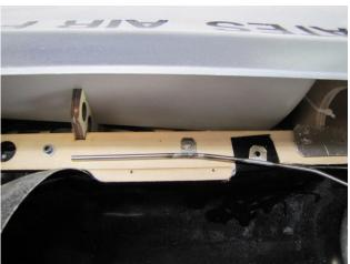
☐ Aim the outlet of the smoke tube down the center of the tail pipe. The long smoke tube reduces the chance of igniting the smoke oil.
