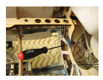
☐ Install the (3) 3mm x 16mm bolts to secure the upper fuse to the lower fuse. A standard 2.5mm hex wrench can be used. The smoke tanks will need to be shifted to gain access to these bolts.
