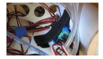
☐ The "GEAR" wire coming from the main controller goes to your Receivers gear channel. The "LED" wire coming from the main controller goes to your Receivers channel of your choice, this will be the channel to control your lights The "LED" channel coming from the RX has three positions, Off, NAV Only, and NAV and Landing lights.
