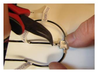
☐ Route the brake line through the hole on the tray and connect it to the open fitting on the brake valve.
