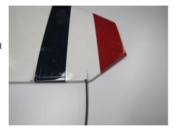
☐ Measure .7" from the edge of the control surface. Mark the cable at this location.
