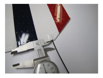
☐ Cut the cable on the mark and then strip 1/8" of the black plastic to expose the cable.
