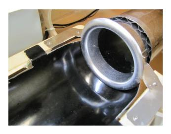
☐ Trim the inlet extension to fit. The final length was 6.875" on this model.
