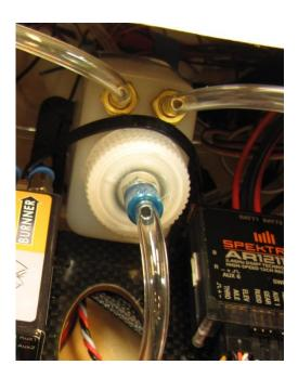
☐ Insert the UAT into the opening provided. Two zip ties are used to secure. The rear zip tie goes through the holes and holds the aft end from rising, while the front zip tie wraps around the board, just aft of the bulkhead.
