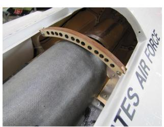
☐ Use Zap-A-Goo to secure the smoke tank to the bulkhead as shown. This prevents the tanks from moving yet allows them to be removed.
