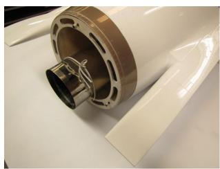
☐ Remove the crossover brace using a 2.5mm hex wrench and pliers.
