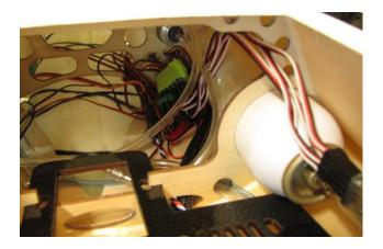
Connect the airlines to the appropriate aluminum "t" blocks. Slide the chrome collar over the tube; slide the tube onto the fitting, slide the collar over the fitting to secure. Do not allow the tubing to slide too far over the barb. Match the labels; Door Closed, Door Open, Gear Up, Gear Down.
