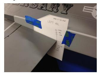
☐ Cut the templates from the last two pages of the manual. Use the heavy paper templates to setup control deflections. Triple rates have been tested. Align the "tick marks" and dashed lines to locate the template onto the fuselage, use tape to secure.
