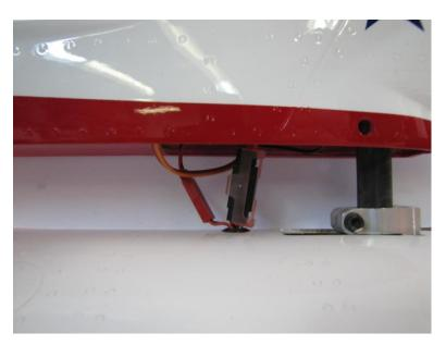
Important! The clamping bolts have "E" clips on the ends of the bolts to prevent the bolt from falling out during transportation. Do not continue to loosen the bolt once you feel the resistance of the "E" clip, you will damage and loose the "E" clip. This is the same on Fin, Stab and Wing mounts.
