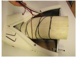
☐ Assemble the lower front fuse to the rear fuse.
