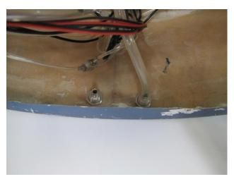
☐ Remove the (2) 4mm x 10mm bolts using a 3mm Allen wrench and the (3) 3mm x 16mm bolts with 3mm washers using a 2.5mm hex wrench.
