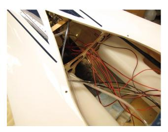
☐ Connect the Smoke Tank Vent hose to the aircraft's right-side vent.
