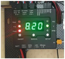
**NOTE**: The **BATT** connection is only used for set up and testing the Black Box when no Receiver Battery is connected. It is not intended to be used in normal operation.
