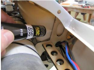
☐ Use Zap-A-Goo to secure the inlet extension to the bulkhead as shown. A dab on either side is sufficient.
