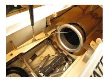
☐ Remove the tailpipe and set aside for installation later.
