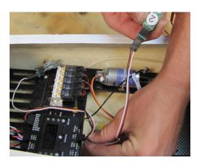
☐ There are (2) three wire servo leads coming off of the light controller modules, plug the servo leads into the "LED" port in the central controller as shown. Make sure the polarity is correct. Both the top and bottom ports are sending out the same signal and voltage.
