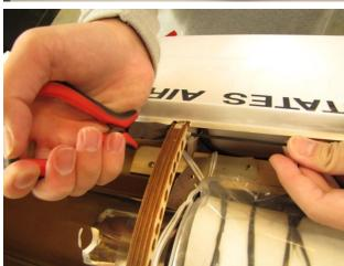
☐ Remove the wire tie securing the tailpipe.
