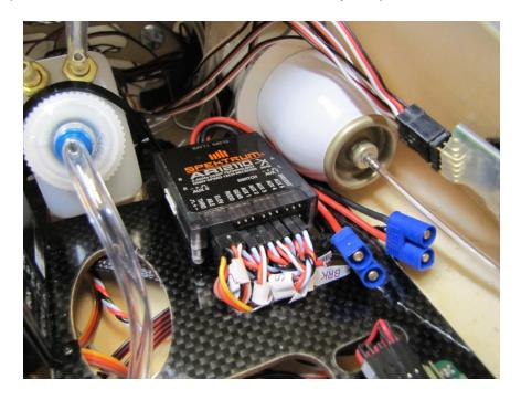
☐ Here are two of the four Spektrum remote receivers mounted in the nose with Velcro.
