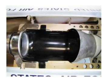
☐ Trim off a small amount until the inlet extension and bypass fit together. Use a sharpie to draw a straight line around the tube.
