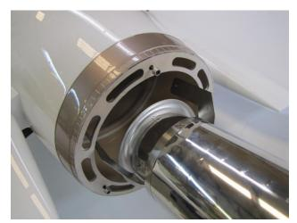
☐ Install the tail cone over the three bolts and twist to lock.
