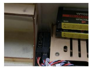
example on a BVM plane used a regular Spektrum 9030 Rx and an X-plus expander. You can find the Rx channel mapping under Connecting Rx wires later in this manual.
