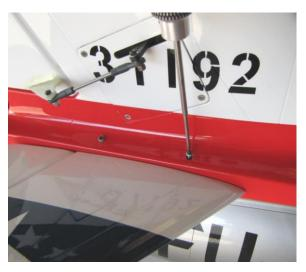
**NOTE**: The elevator neutral position is located as shown.
