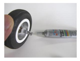
Reassemble the wheel, brake, and axle. Use a small drop of thread locker on the set screw. Check for free spin of wheel and brake application.
