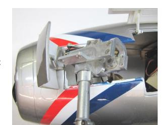
☐ Maneuver the retract unit to get it out of the model. Use a BVM Collar Tool to disconnect the pneumatic lines from the nipples on the cylinder.
