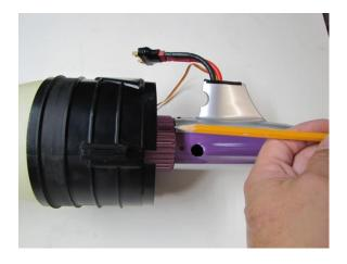
If the spinner is rubbing on the spike, you can use a sanding block to remove the flange on the back of the spike.
