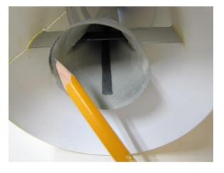
□ When mounting the fan, slide the intake into position, then slide the fan onto the inlet. This will become the location for your fan to sit. Use a 1/16 drill bit to mark the location of the mounting holes.
