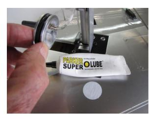
Apply super axle lube to the axle from inside and outside access. Note the nylon spacer.
