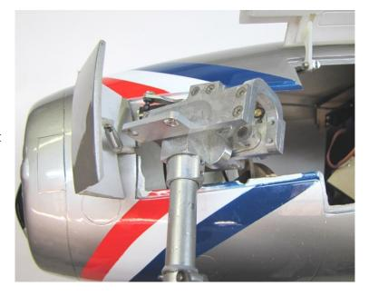
NOTE: The steering arm linkage may differ from that shown here. Disconnect the steering linkage from the steering arm.
