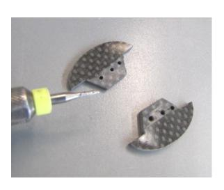
☐ Use ZAP-RT or similar rubberized glue to attach the Skidz as shown. Wipe away excess before it cures.
