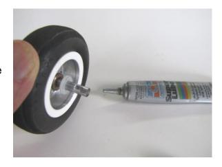
Reassemble the wheel, brake, and axle.
