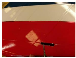
☐ Use a 1/16" Carbide Cutter to add some glue holes as shown.
