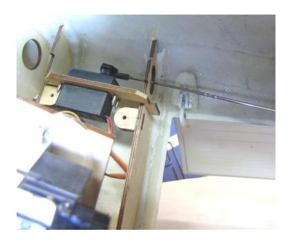
☐ Lift the servo mount up as shown. The wire linkage should slide out of the slot in the #3 bulkhead. The servo could be changed with this access.
