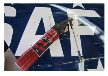
The wings are retained to the fuse with (2) 3mm X 25mm front and (2) 3mm X 16mm screws at the rear. Use a 2.5mm hex wrench.
