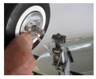
□ Apply Parker Super "O"Lube to the brake "O"Ring and on wheel inner drum.
