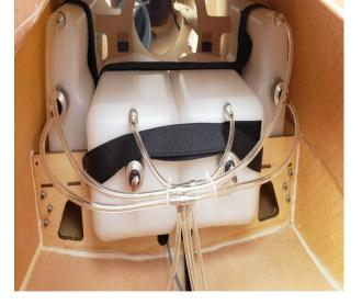
On the BVM demo model we use a 6mm ball valve (BVM # 5315) at the Smoke tube to stop the smoke from dripping into the Pipe during fill up and shutdown.
