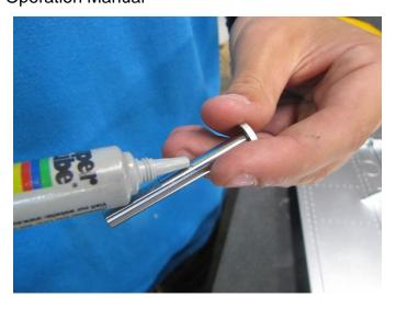
Once all parts have been Lubed and Greased. You can reassemble using the above steps. A small amount of Pacer Z-42 Loctite is used on the Axle Set Screws.
