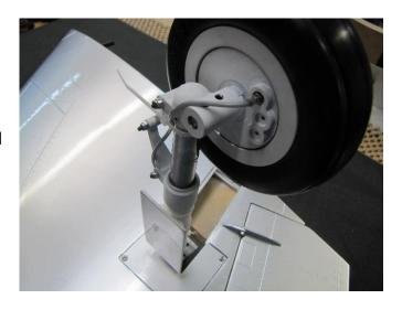
☐ Remove the (3) Philips head screws. This will allow you to remove the plastic wheel cover and remove the Axle.
