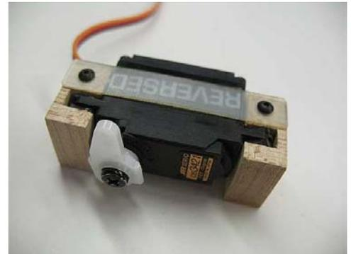
Note: A reverse servo is required on either the rudder or nose gear steering unless two channels are used and mixed.
