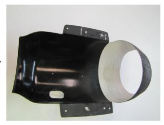
☐ Use a Dremel "dish" cutter or similar tool to bevel the upper inside edge of the engine mounting rails to accept the Bypass.
