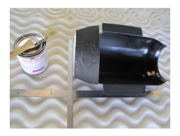
☐ Drill (2) 3/32" holes in the bottom of Bypass to allow a fuel spill to drain out. Make a clearance hole for the fuel line hook up to the engine. This may not be necessary for some engines.
