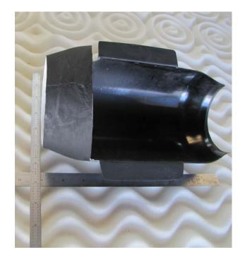
☐ Scuff the inside aft section with medium sandpaper or a 3M #7447 red scuff pad. Brush-on 3 coats of BVM "Heat Shield" (BVM# PA-MA-1940).
