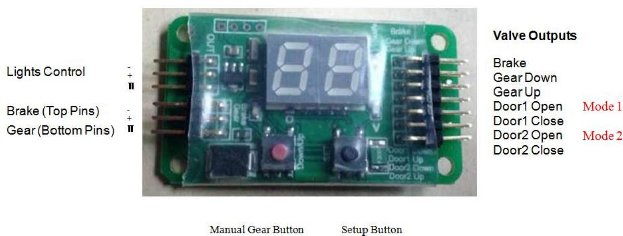
This extremely simple sequencer includes 2 modes of gear/doors sequence, and brake and landing light control. The sequencer features push button programming operation for sequence timing and low pressure failsafe protection.
