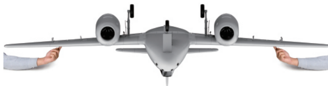
A general method for measuring the center of gravity
