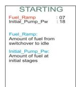
There are only two adjustable parameters in this sub-menu, "Initial pump Pw" values and "Fuel Ramp".
