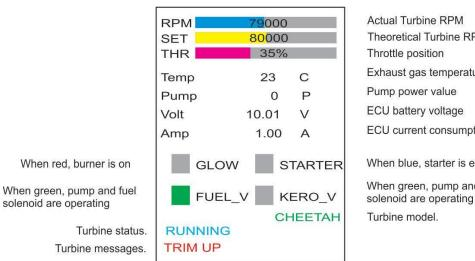
**Theoretical Turbine RPM** Exhaust gas temperature ECU current consumption When blue, starter is engaged When green, pump and burner
