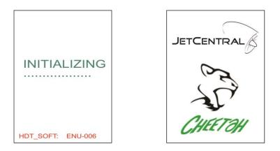
When the POWERPACK / ECU is connected to the HDT, the ECU battery is connected and the RX power is turned on, the HDT display screen will briefly display "INITIALING" with the software version of the HDT displayed across the bottom of the display, and then briefly displays the Logo of the turbine that is connected, after a few seconds the main screen will be displayed.
