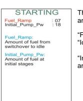
There are only two adjustable parameters in this sub-menu, "Fuel Ramp" values and "Initial Pump Pw".
