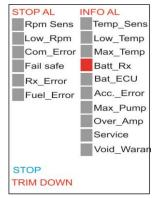
Stop Alarms appear when the problem was significant enough that the ECU command the turbine to stop during a run cycle.
