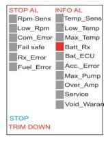
"Temp\_Sens" indicates a temperature probe failure.
